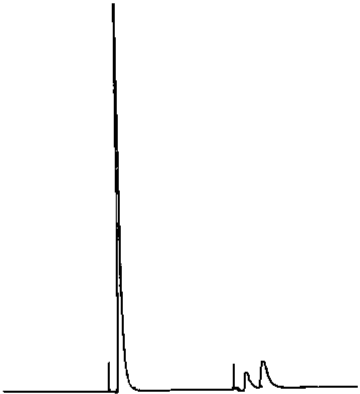
Chromatogram 2. The ion chromatograms: a - sample, anolyte medium 1:200; b - standard ( \text{ClO}_3^- ) with concentration 29.5 mg/l.
