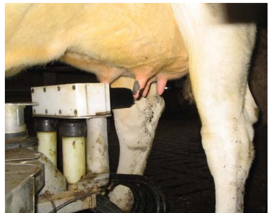
Brushes on the robot are disinfected with ANK
