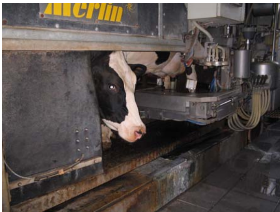
Brushes on the robot are disinfected with ANK
